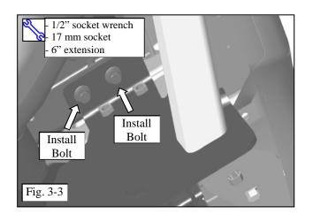
Install Bolts Fig.4-1 Install Bolts - 1/2" socket wrench - 17 mm socket - 6" extension
