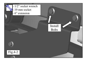
(c) Install two (2) M12 bolts through the 14 x 20 mm slots on the tie plates, into the bottom of the frame on both sides (LH/RH) (Fig. 3-3).
